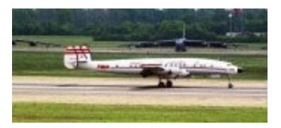
The vertical stabilizer usually is a single panel extending upward from the aft fuselage. Exceptions to the single-panel rule include twin vertical stabilizers used on the Twin Beech and Skymaster. It's a popular configuration on military airplanes such as the F-15 and F/A-18. Triple vertical stabilizers also have been used, most famously on the Lockheed Constellation. In each instance, their job is the same: to minimize and control the airplane's rotation about its vertical axis.
